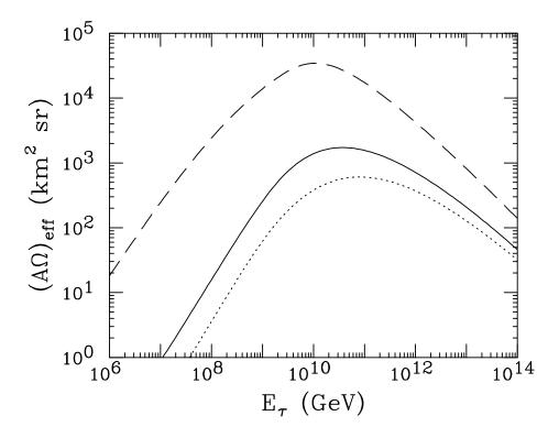
Effective apertures at Fly's Eye (dotted), HiRes (solid), and Telescope Array (dashed).
