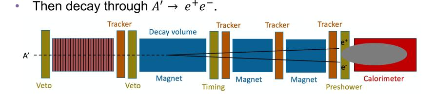
The signal is no charged particle passing through the upstream veto scintillator detectors, followed by two very energetic (100s of GeV) charged tracks in downstream trackers. Tracks are very collimated, but magnet splits them sufficiently to be seen as 2 tracks in trackers.
