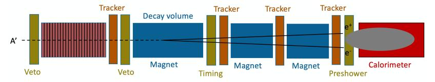
The signal is no charged particle passing through the upstream veto scintillator detectors, followed by two very energetic (100s of GeV) charged tracks in downstream trackers. Tracks are very collimated, but magnet splits them sufficiently to be seen as 2 tracks in trackers.
