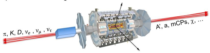
Solution: the LHC is a circular collider! If we go far enough away, the LHC proton beam will curl away, while all the light, weakly-interacting particles we are looking for will go straight.
