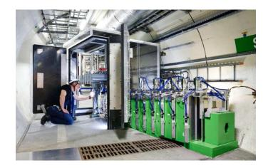
The new experiment SND@LHC installed at CERN's Large Hadron Collider. Neutrinos impinge on the detector from the left and interact
