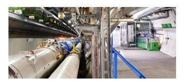
A section of CERN's Large Hadron Collider (left) and the new experiment SND@LHC (right). Neutrinos are produced at one of the LHC's collision points, hidden behind the curvature of the accelerator, and interact in the SND@LHC detector after traversing around 100 meters of rock and concrete. Credit: Brice, Maximilien; SND@LHC Collaboration.
