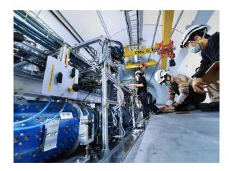
The final elements of the FASER (Forward Search Experiment) detector are installed in the TI12 tunnel of the LHC. It is located along the beam collision axis, 480 m from the ATLAS interaction point, in an unused service tunnel that previously connected the SPS to the LEP collider. FASER began taking data in July 2022 at the beginning of LHC Run 3. Photograph: Maximilien, Brice; Ordan, Julien, FASER Collaboration.
